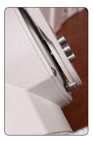
Photo shows Stop Block pushing against the switch lever arm.
