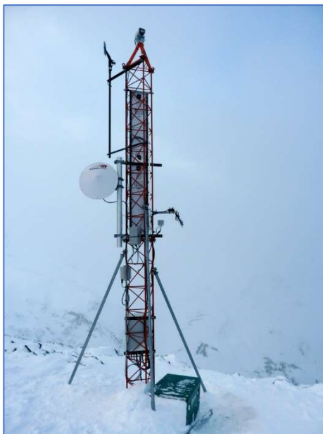
JPTH-13MPoE Positioner on Top of a Weather Instrumentation Tower in the Canadian Rockies - Canada
