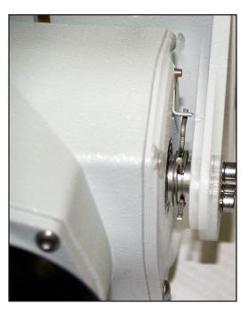
Photo shows tilt actuator tripping the switch lever arm.
